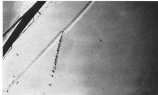
Figure 6 Array of etch-pits forming a tilt boundary in GaSe. The short array of pits denotes a slip trace ( \times 108 )
